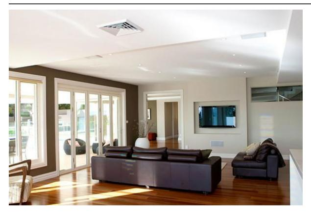
Reverse Cycle Ducted Air Conditioning System provide discreet air conditioned comfort throughout your entire home. The ducted system can be installed in a new home or tailored to suit an existing one, and once installed only the controller, the return air grill and discharge vents are visable inside your home. With up to 60 months payment options\*, there will never be a better time to call Climat for a quote.
